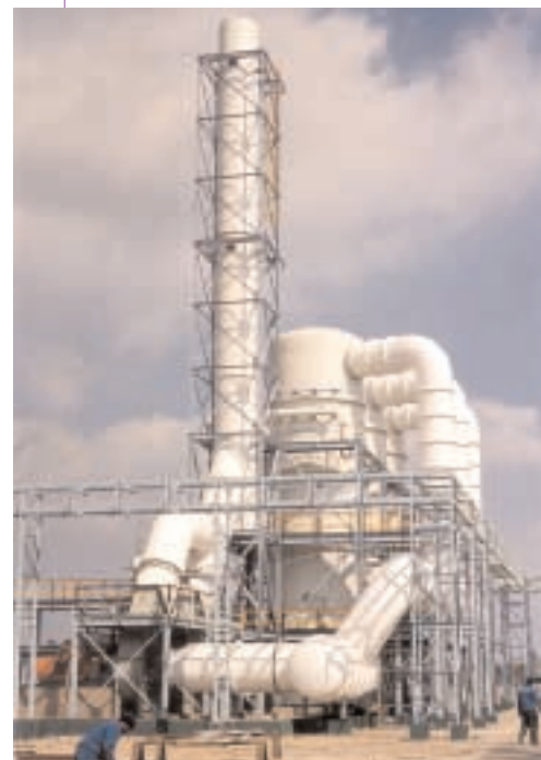
This scrubber assembly was manufactured with VE8300 resins.
