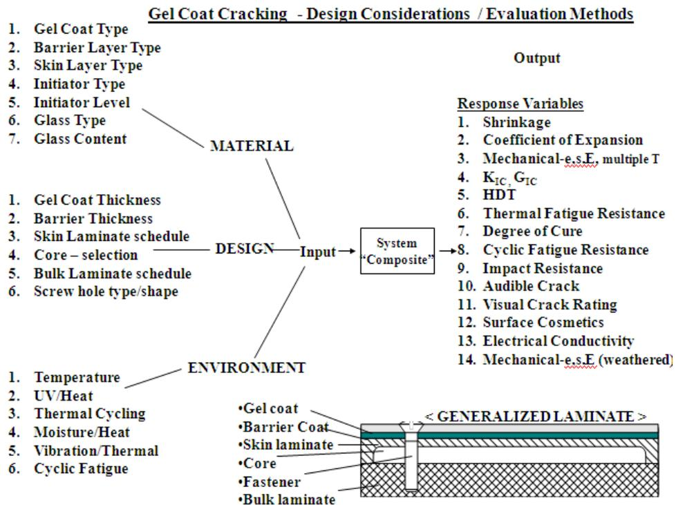
Standard test methods are available from ASTM (D-638, D790) and others for determining the flexural strength, tensile elongation and other mechanical properties of bulk resin or gel coat castings. The ASTM methods subject thick castings (0.25 inches) of the gel coat to controlled strain levels in a universal testing machine (ex. Instron, MTS).
