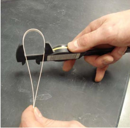
Record the thickness and fail diameter of each strip in a spreadsheet for calculation. Use the equation below to calculate the percent elongation for each strip. Calculate the mean elongation of the 15-25 strips and calculate the standard deviation. If the standard deviation is less than 10% of the mean value, the test can be considered valid. If the standard deviation is more than 10% of the mean the variability is too high and the results should be discarded.
