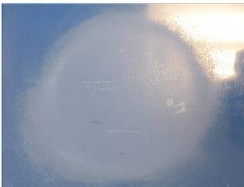
Continue this spray pattern until the patch area is thoroughly covered with gel patch. Sufficient patch gel coat should be applied to the repair area such that the cured patch can be sanded and buffed to the level of the surrounding, non-repaired area.
